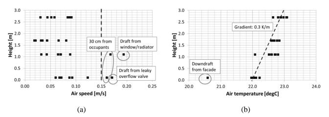
Figure 7. Air velocities (a) and air temperature (b) at different heights in renovated classroom 15.
