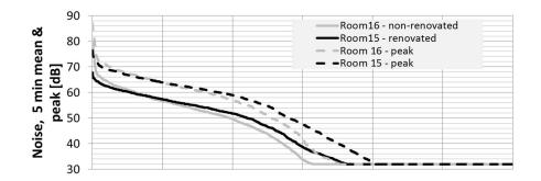
Figure 5. Sorted mean and peak noise levels in renovated and non-renovated classrooms in March.
