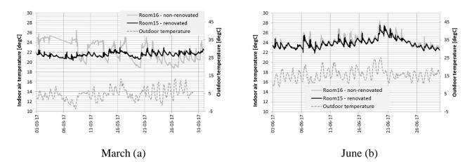
Figure 4. Indoor air temperature in March (a) and June (b) in the classrooms (solid lines, left y-axis) along with the outdoor temperatures (dashed line, right y-axis).
