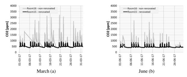
*Figure 3.* CO<sub>2</sub>-concentration in March (a) and June (b) in classrooms 15 (renovated) and 16 (non-renovated).
