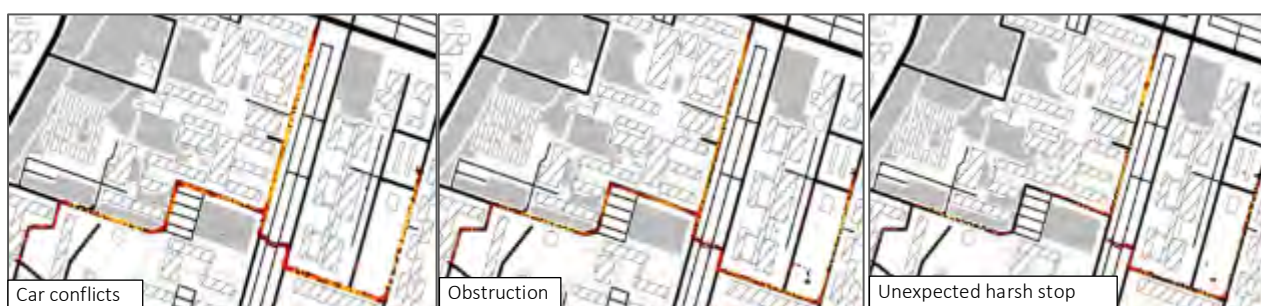
MAP 8.3 A–C SHUTTLE SPEED WHEN EVENT REGISTERED. 0–15 KM/H: DARKER COLOURS INDICATE LOW SPEED, BRIGHTER COLOURS INDICATE HIGH SPEED.
